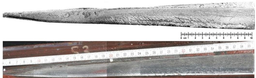
**Figure 4.** Magnetic particle inspection (above) and camera (below) images of the rolling surface on a frog nose after 33 Mt [26].
