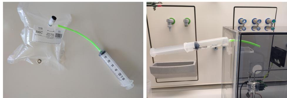
**Figure 6.** Small volume gas sample testing <1 L.
