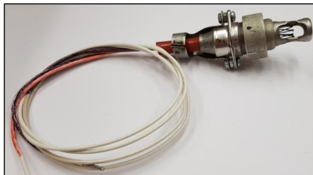
Figure 1. View of the DPS transmitter.
