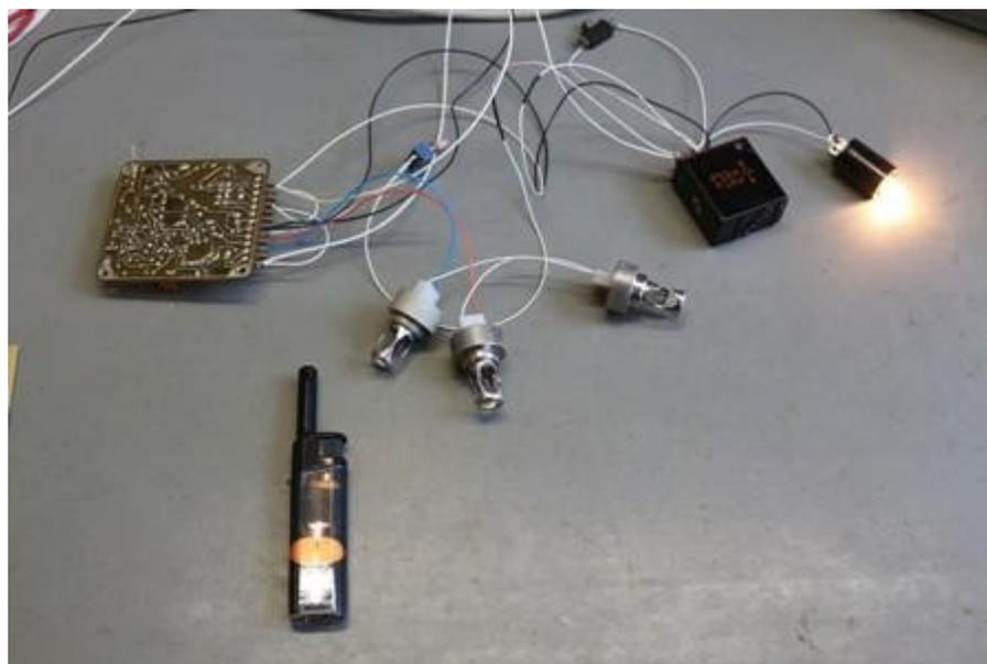
**Figure 13.** View of the measuring system for testing the block for disturbances in the supply voltage.
