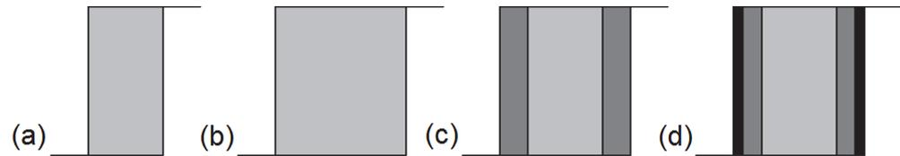
**Figure 3.** Possible approaches to addressing the change in hysteresis shape at increased excitation frequency: (a) quasi-static hysteresis loop, (b) dynamic hysteresis loop, no distinction is made as far as dissipation mechanisms are concerned, (c) hysteresis loss is distinguished from eddy current loss, (d) dynamic loss partitioning into classical and excess terms (following e.g., Bertotti’s approach [33]).
