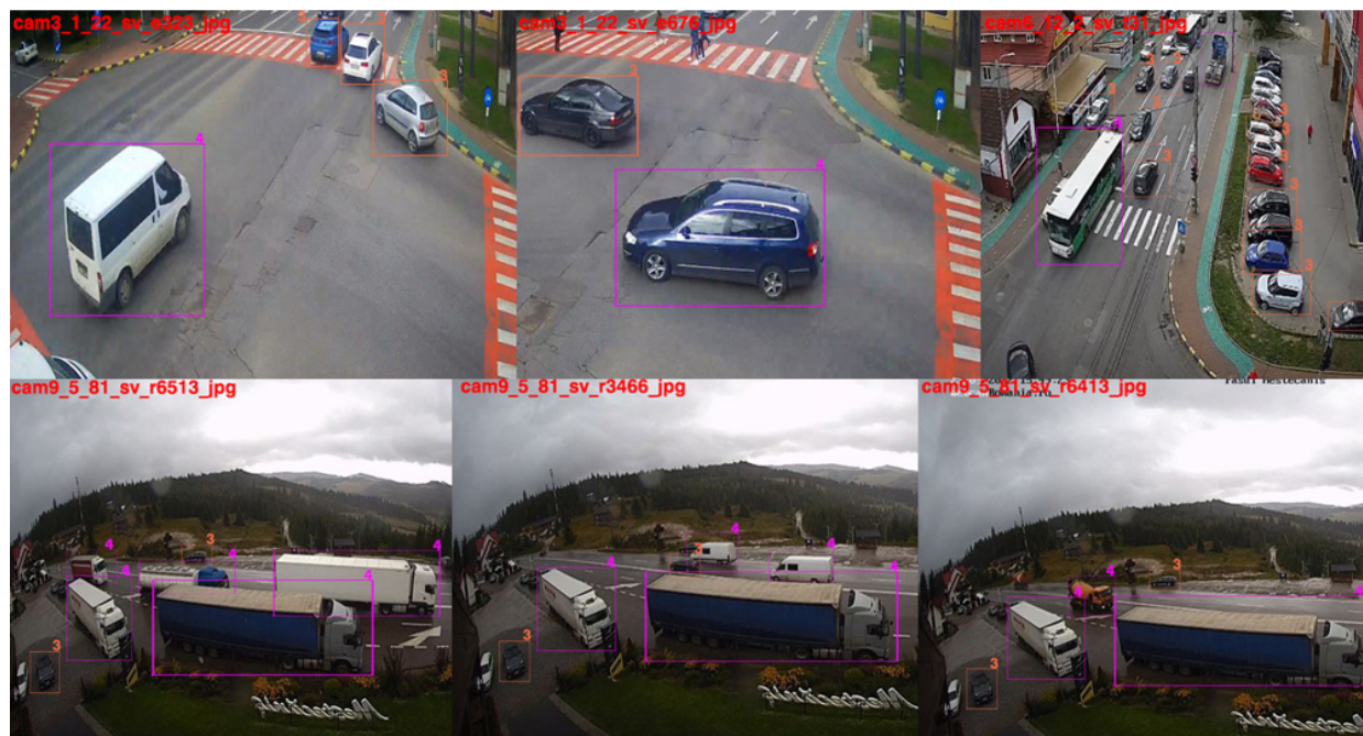
Figure 8. Analysis of the results obtained for the YOLOv5r training model using the SR1 test dataset. Analysis of established classes for vehicles, buses, taxis, bicycles, trucks, vans, auto-trucks.
