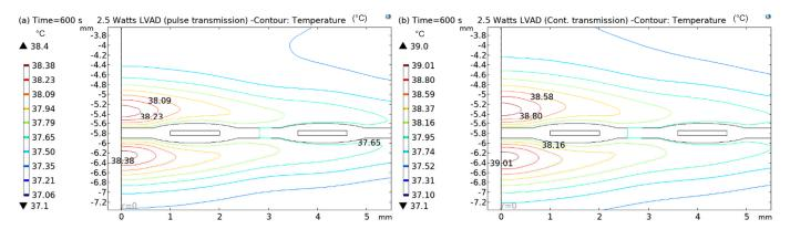
**Figure 13.** Contour plots of thermal analysis: (**a**) pulsed and (**b**) continuous transmission modes for 2.5 W LVAD.
