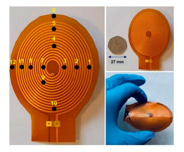
**Figure 3.** An illustration of thin and flexible coils with the position of the twelve NTC thermistors (numbered 1 to 12) adhered on the coil surface.
