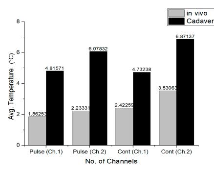
**Figure 11.** Maximum average temperature changes for in vivo and cadaver measurements at 5 W LVAD under pulsed and continuous transmission protocols (channel 1 and channel 2).
