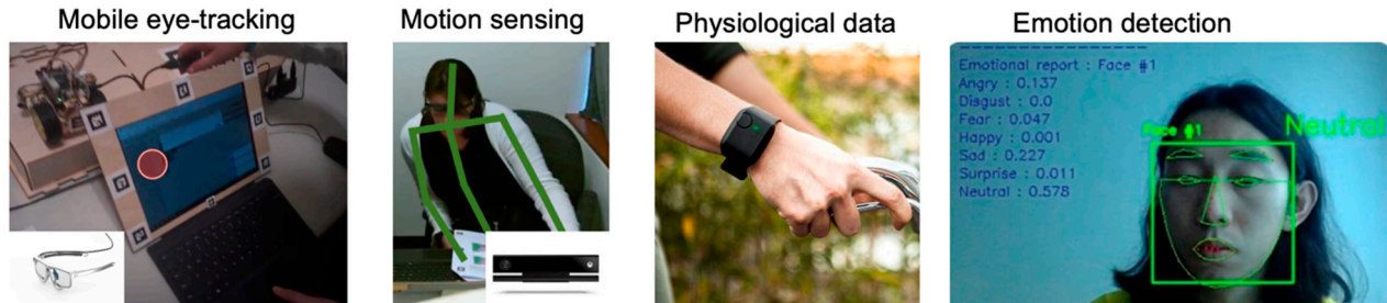
Figure 1. Use of sensors in a typical multimodal study. Left: mobile eye-tracker. Middle: Motion sensors and Electrodermal wristbands (Empatica E4). Right: emotion detection from facial expressions. Mobile eye-trackers are expensive wearable sensors and data processing software tend to be proprietary. The Kinect sensor is more affordable but does not come with an easy-to-use data collection package; recording the data requires some programming knowledge. The Empatica E4 is also relatively expensive and data extraction requires proprietary software.
