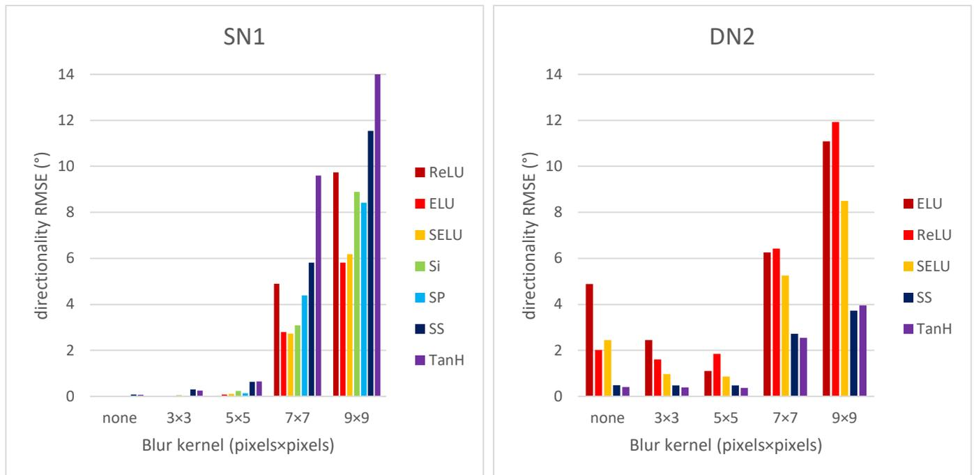
**Figure 7.** Directionality RMSE for CNNs SN1 and DN2 vs. blur kernel size.
