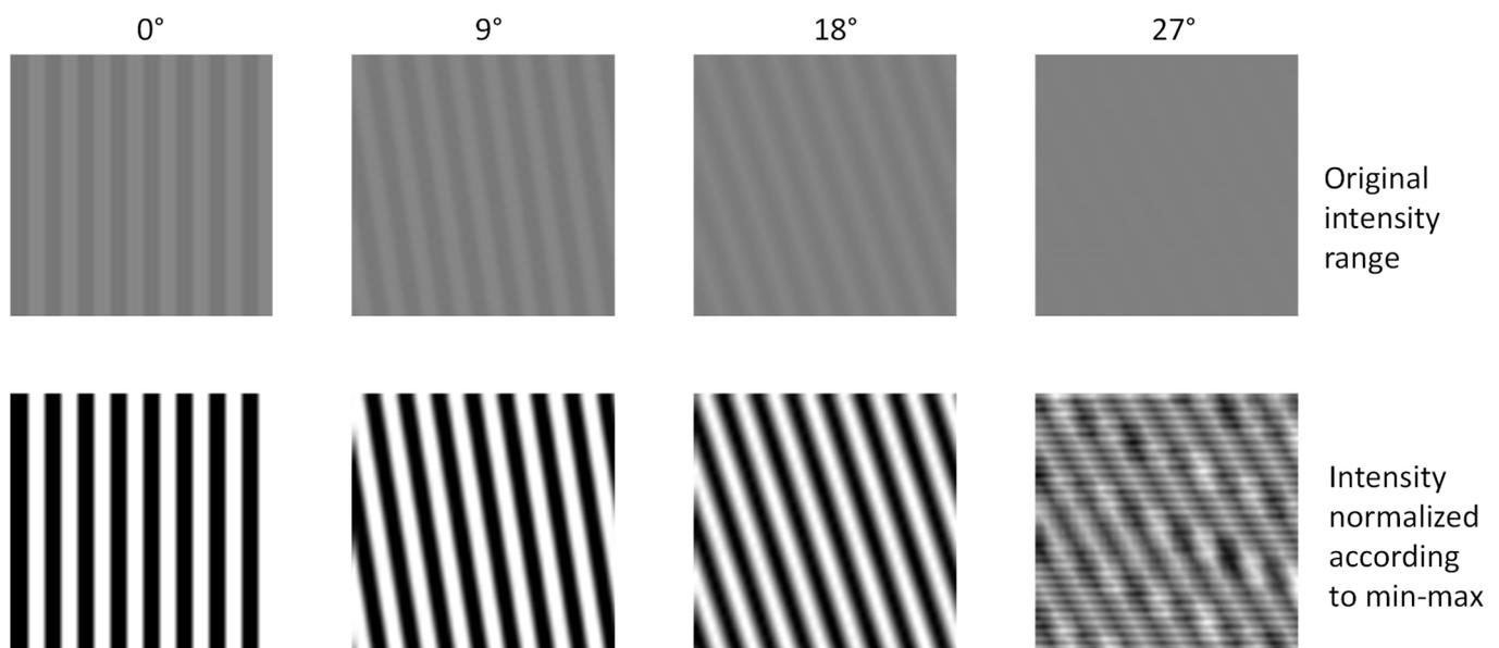
**Figure 11.** Instance of bars of bar size 4, bar period 8 and blurred by averaging filter with kernel size of  $9 \times 9$ .
