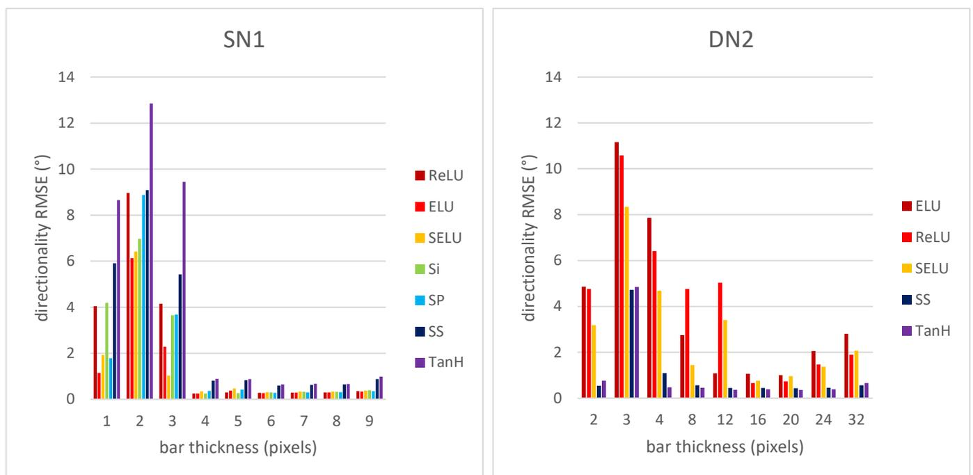
**Figure 6.** Directionality RMSE for CNNs SN1 and DN2 vs. synthetic texture bar thickness.
