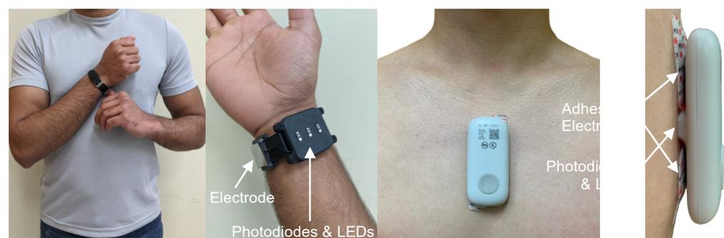
**Figure 10.** Device form factor. Electrodes for a single-lead ECG, photodiodes and LEDs to record the PPG, and tri-axial accelerometers and gyroscopes (internal to the devices) to acquire the SCG signal can be customized and modularized to work in multiple form factors. The left side shows the watch-based approach described in [60], while the right side shows an updated version of the chest-worn patch originally described in [59].
