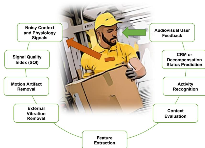
**Figure 15.** Processing stages in an example use case. Noisy signal recordings from a ruggedized chest-worn sensor (brown) go through a signal quality assessment and then motion and external vibration removal prior to feature extraction. Once high-quality features are extracted from the signals, predictions and evaluations of context, activity and reserve or decomensation status can be made. This summarized information is then relayed back to the user.
