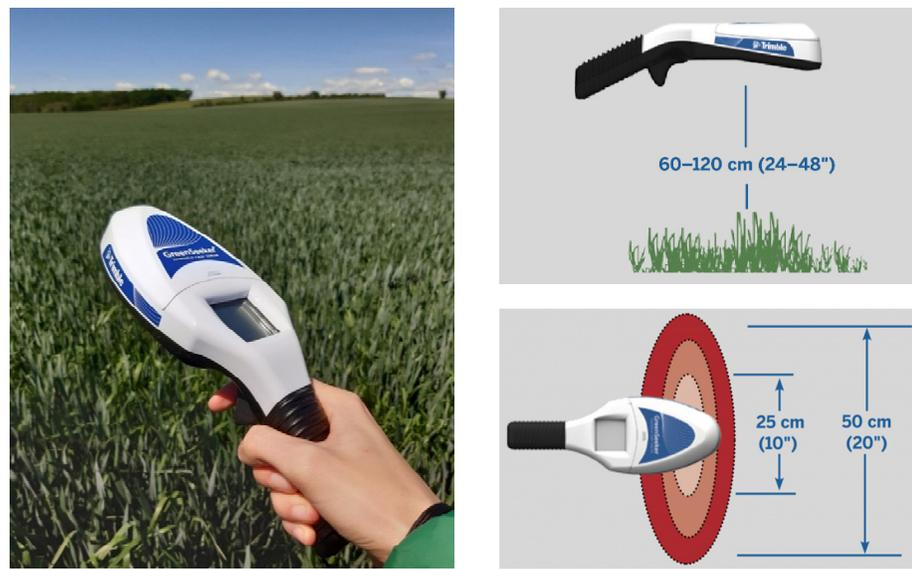
**Figure 1.** (Left) GreenSeeker spectrometer for ground measurements (photo: Paulina Raeva), (right) functionalities during NDVI field measurements
