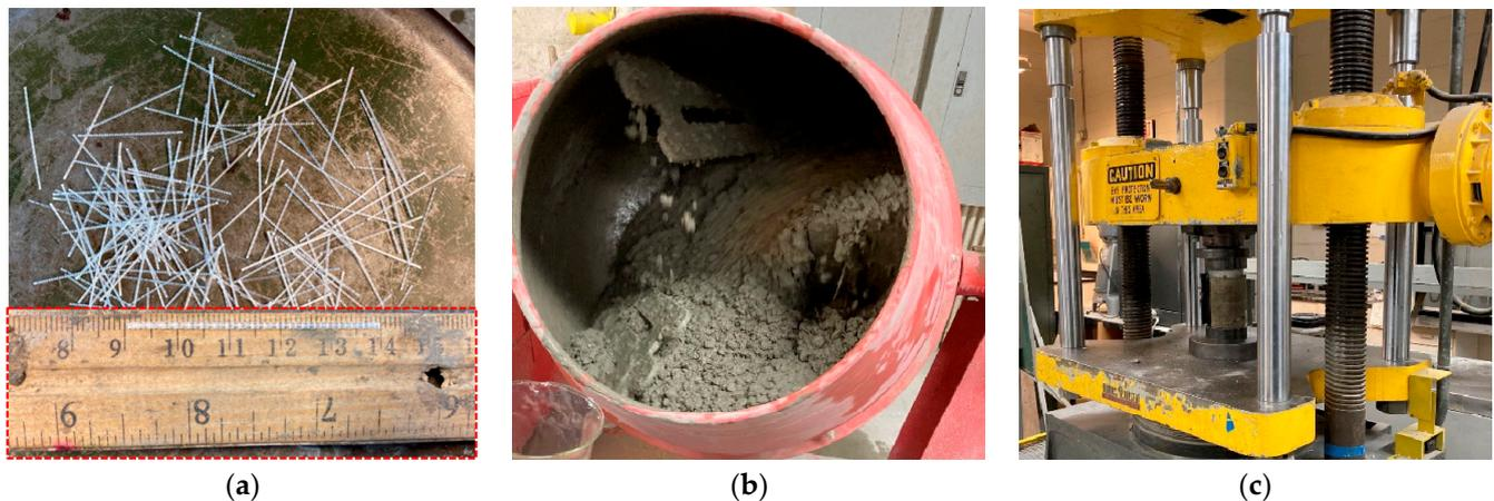
**Figure 1.** (a) Fiber appearance and fiber length of 50 mm; (b) concrete mixture in a mixer with a capacity of 170 L; and (c) compressive test for cylinder concrete specimen.
