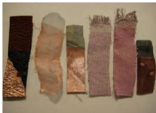
**Figure 3.** Different textile conductive materials for flexible antennas. Reprinted from ref. [15].
