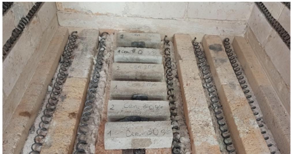
**Figure 2.** Samples during annealing at 300 °C.
