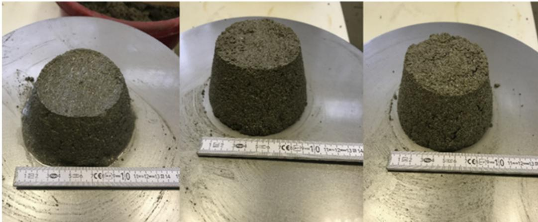
**Figure 4.** Consistency test—from left to right, 10, 20, and 30% MCC mortars.
