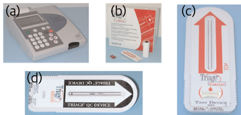
Figure 8. Alere's Triage® system based on fluorescence immunoassay. Photographs of the reader (a), the LFIA used for quantitative analysis (b,c), and the QC device used for quality control (d) are shown.
