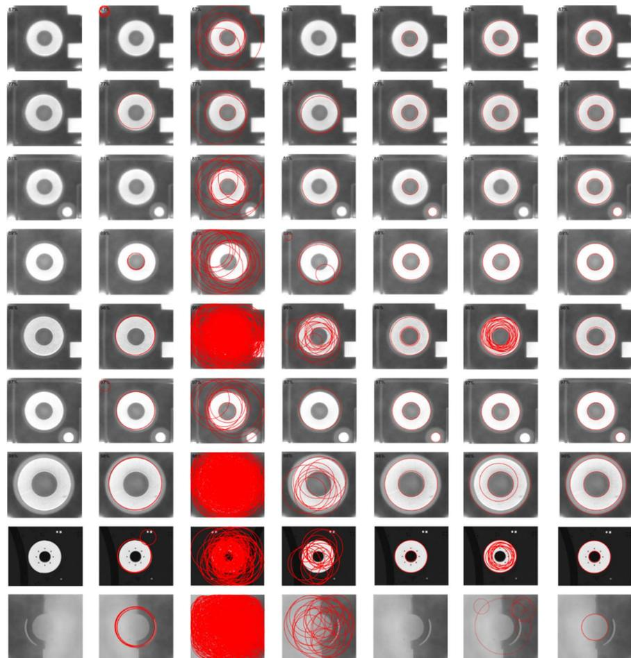
**Figure 9.** Circle detection results on the dataset PCB, which is widely used by other algorithms. From the left to right columns: input image, RHT, RCD, CACD, Jiang, Wang and ours. As can be seen, the proposed method obtains better performance than the others.
