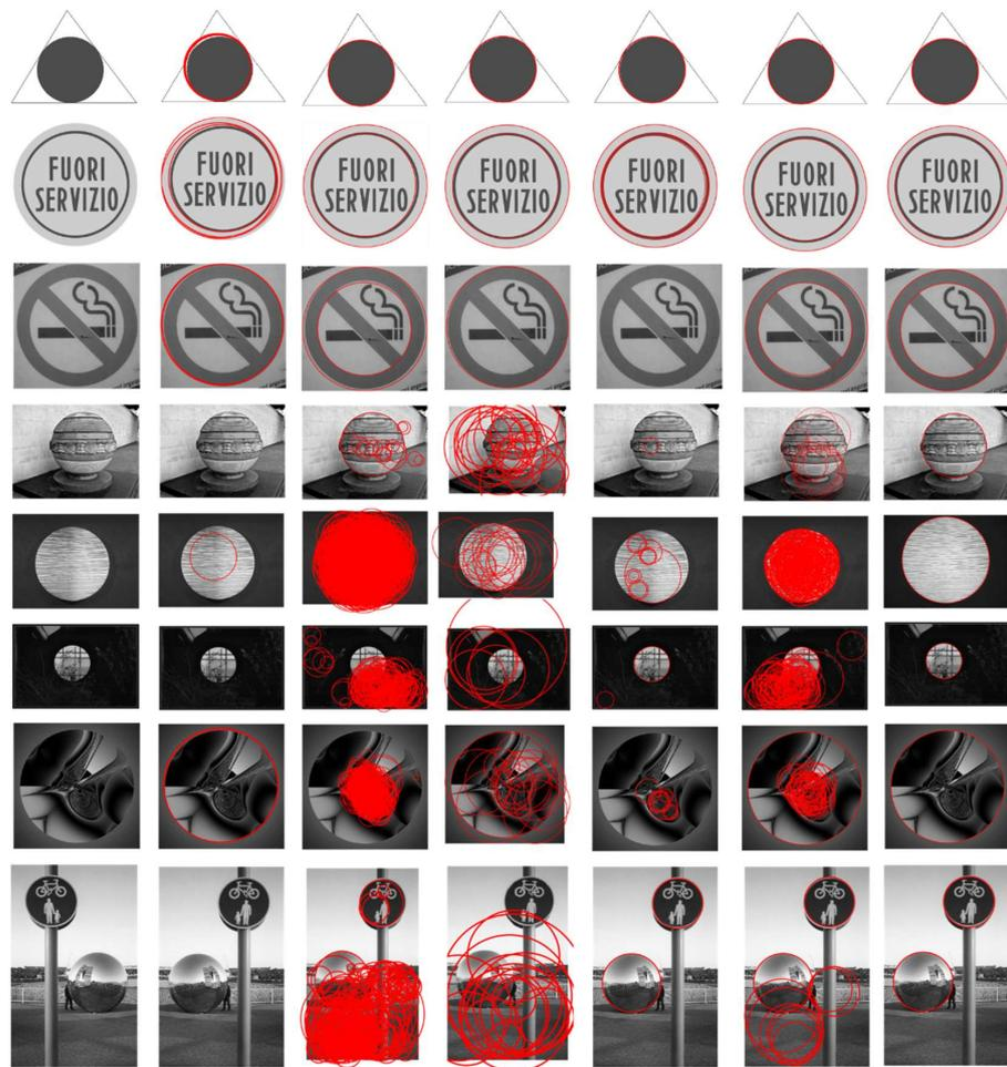
**Figure 8.** Circle detection results on the dataset GH, which is widely used by other algorithms. From the left to right columns: input image, RHT, RCD, CACD, Jiang, Wang and ours. As can be seen, the proposed method obtains better performance than the others.
