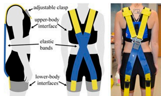
Figure 4. Bio-mechanically-assistive garment prototype [57]. Reprinted with permission from IEEE. License Number: 5383600890958; license date: 7 September 2022.
