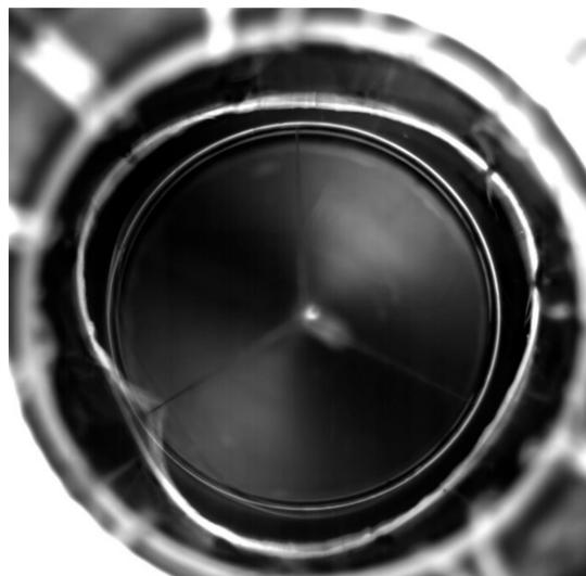
(a) Collapsing morphology (Buckling modes visible) at  $t = 1$  ms.
