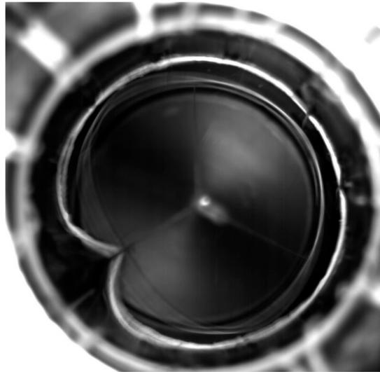
(b) Collapsing morphology (Buckling modes disappear) at  $t = 2$  ms.
