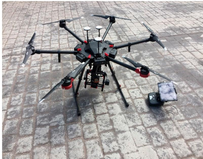
**Figure 2.** UAV DJI Matrice 600 and WIRIS Pro dual sensor used for image capture.
