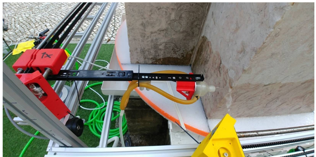
Figure 12. Zoom of the system expelling the waterjet from the pipes to the nozzles and inspecting the base of the column.
