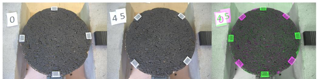
**Figure 8.** Triplet image. **Left:** 0th position. **Centre:** 45th position. **Right:** Overlapped before transformation.
