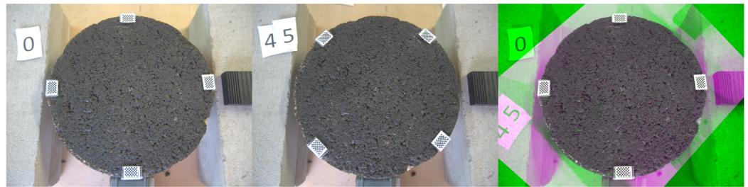
**Figure 10.** Triplet image. **Left:** 0th position. **Centre:** 45th position. **Right:** Overlapped after transformation 45th  $\rightarrow$  0th.
