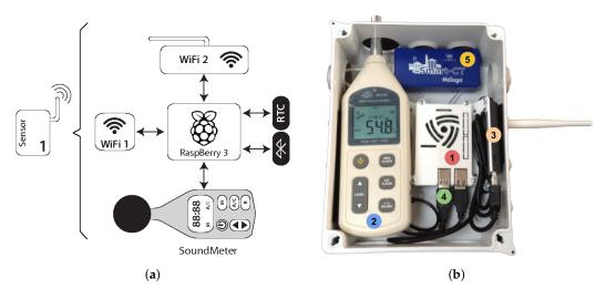
**Figure 2.** Different elements and views of the road sensor system: (a) Sensor block diagram; (b) Actual photo of the sensor.
