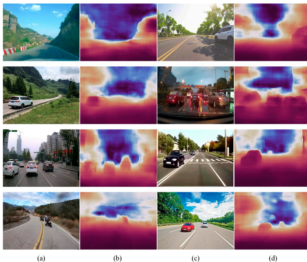
Figure 10. Depth estimation results of the proposed method on the collected road samples. (a,c) Images from the internet; (b,d) proposed method.
