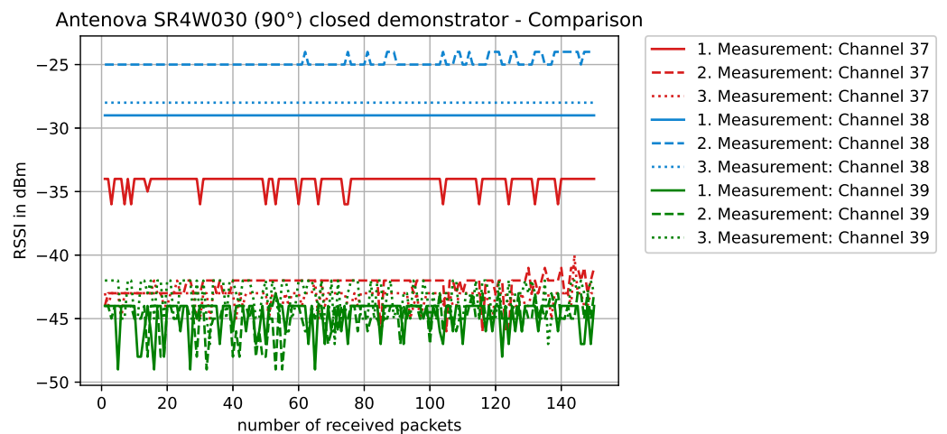
Figure 15. RSSI values with antenna SR4W030 at position 4 with the experimental testbed's lid shut. The antenna is rotated 90° and the antenna structure is normal to the front panel.
