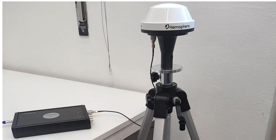
**Figure 4.** Setup used for the experimental dataset collection: Septentrio PolarRx5 receiver connected to an A42 Hemisphere antenna.
