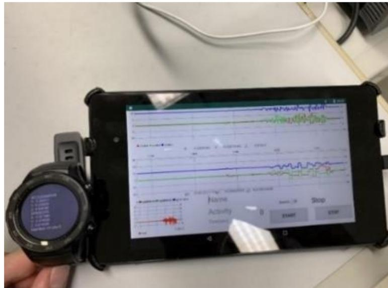
**Figure 1.** Huawei Watch 2 and tablet. The waveforms transferred from the device are displayed and recorded on the tablet.
