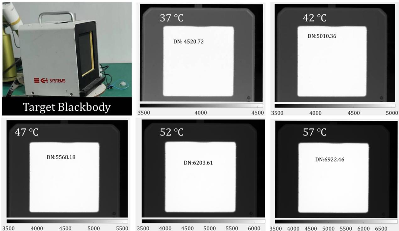
**Figure 9.** Target blackbody and its imaging at different temperatures.
