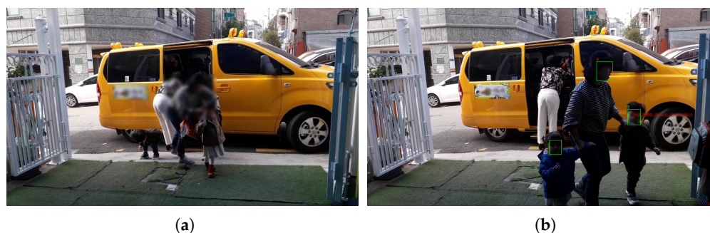
Figure 6. Images taken with a camera installed at the school bus traffic stop (Figure 4c): (a) example; (b) recognition result.
