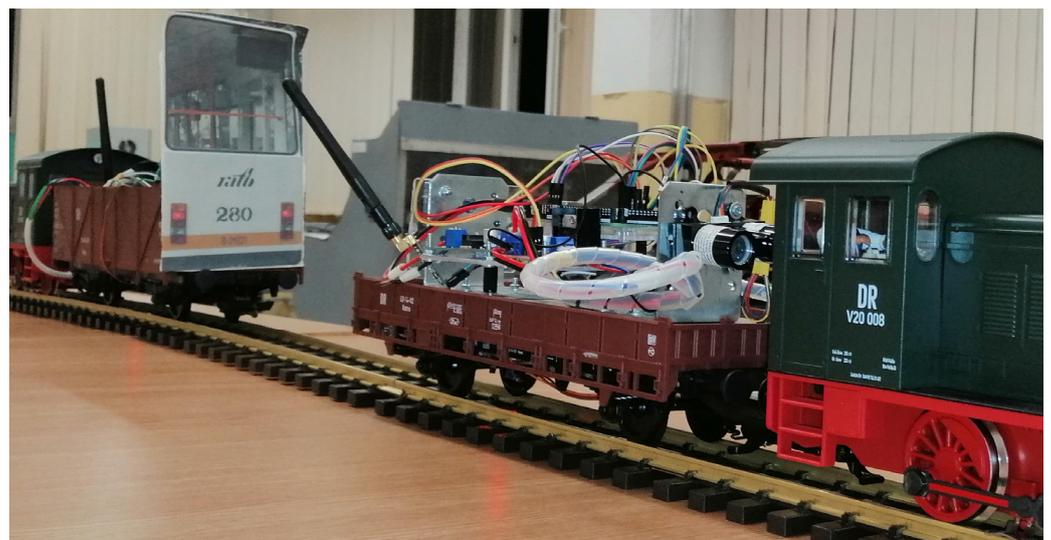
**Figure 1.** Scaled tram model for indoor testing of long-range LiDAR.
