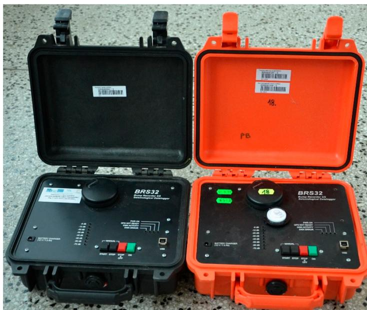
**Figure 1.** BRS32 seismic stations used as reference meters.
