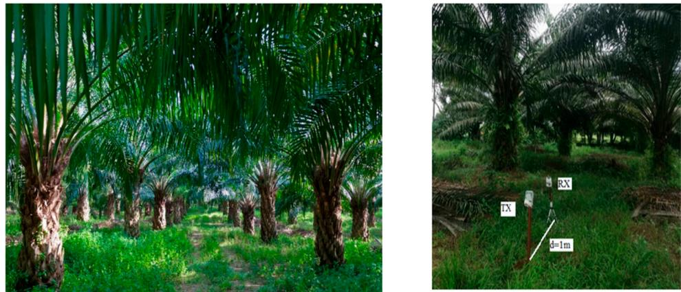
**Figure 5.** LOS links in between the two lines of trees (left); RSSI measurement (right).
