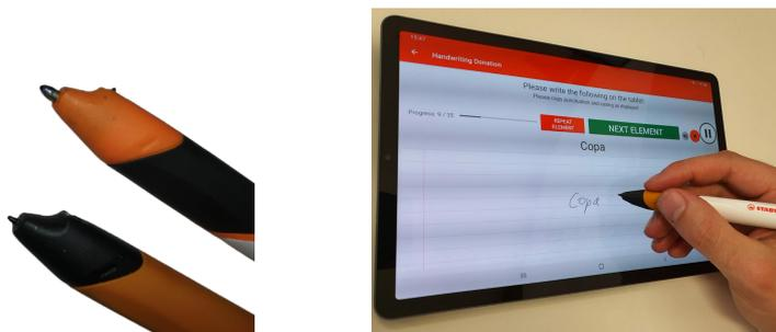
**Figure 3.** Wacom compatible writing tip on the Digipen (left bottom pen), and the recording app (right).
