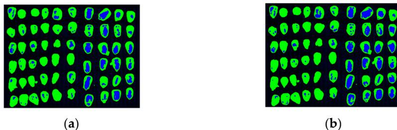
**Figure 13.** Classification results of SVM and LDA in corn kernel mildew hyperspectral image data (spectral and image features) (a) SVM and (b) LDA.
