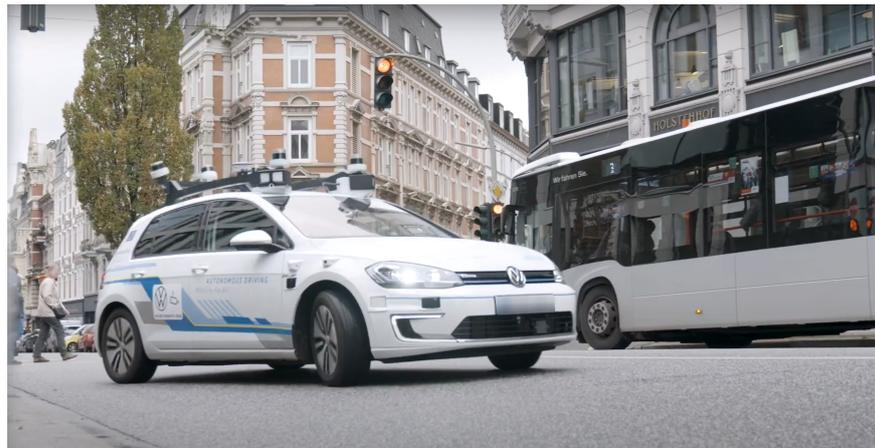
**Figure 1.** The UP-Drive demonstrator vehicle, based on a VW eGolf, navigates urban environments in fully automated mode at the completion of the project.
