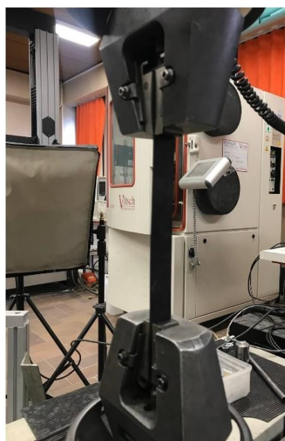
Figure 8. Unidirectional tensile test performed on rubber samples with different curing times.
