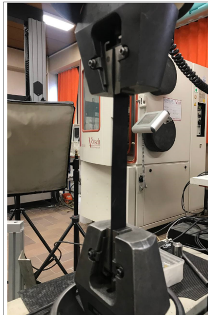
Figure 8. Unidirectional tensile test performed on rubber samples with different curing times.
