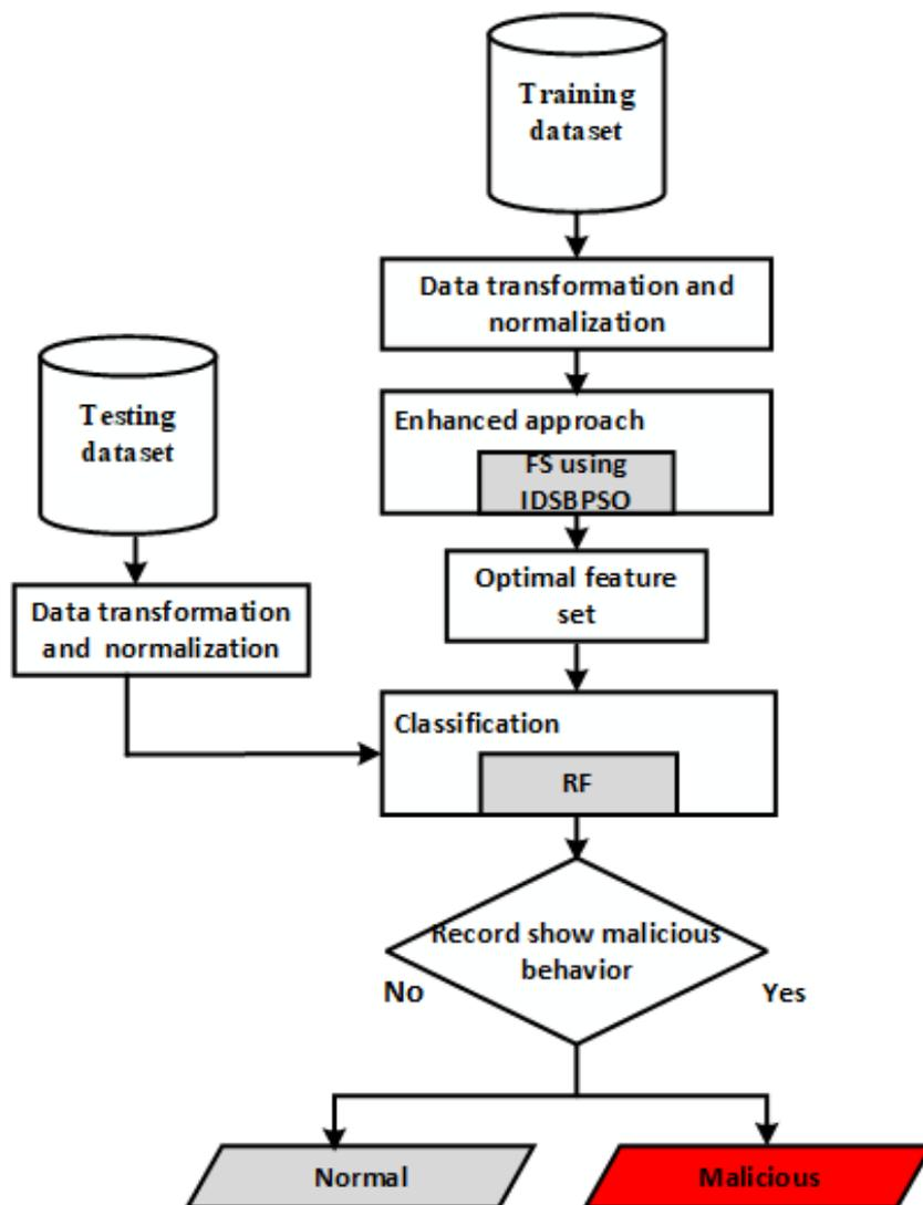
Figure 3. Working architecture of enhanced IDS, using IDSBPSO.
