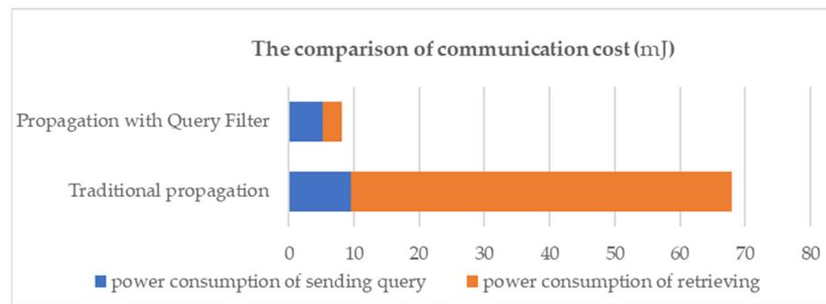
**Figure 9.** The power consumption of query with and without a query filter.
