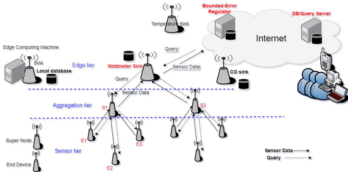
**Figure 2.** System architecture of an edge-computing OBEQ for IoT (S1, S2 are SNs, E1–E3 are EDs).
