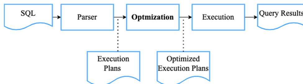
Figure 1. The flowchart of an SQL query process.
