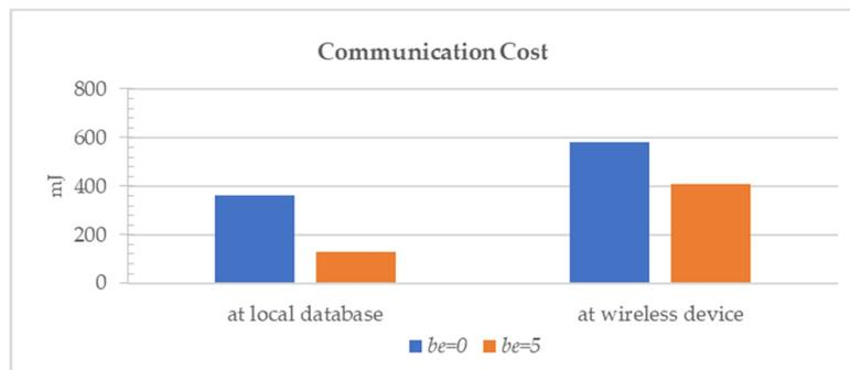
Figure 12. Communication cost of a query with fundamental operations.
