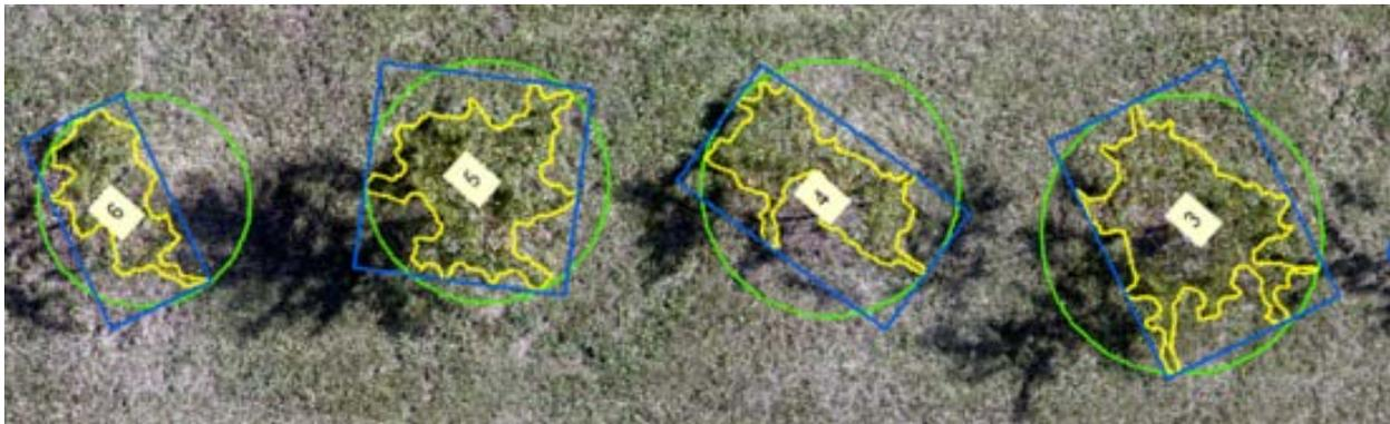
**Figure 3.** Individual tree boundary (polygon, bounding box, and circle) used to extract the tree height and canopy crown volume.
