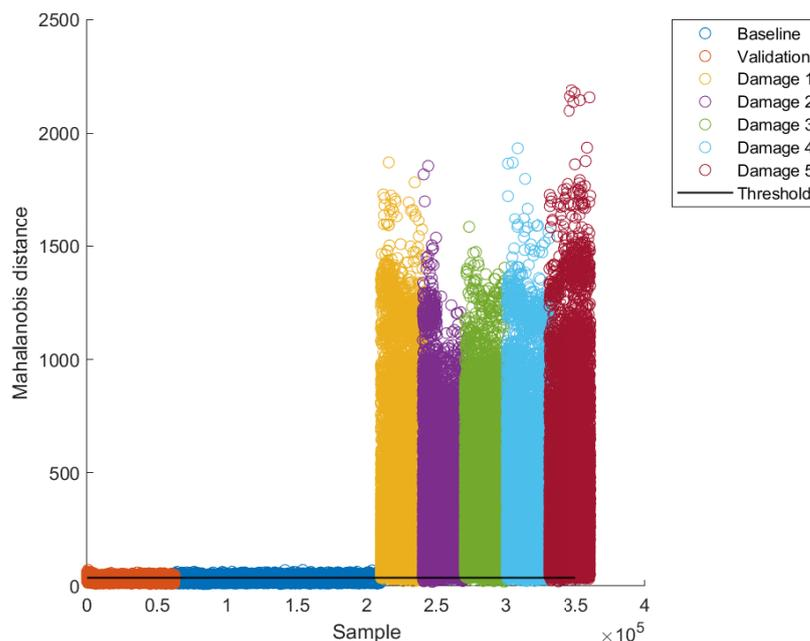
**Figure 14.** Results for an excitation frequency of 17.5 Hz with optimum threshold.
