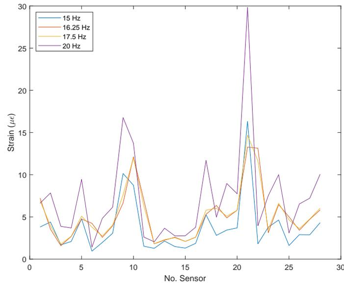
**Figure 8.** Strains for pristine condition versus sensor number (FBG number) for all excitation frequencies.
