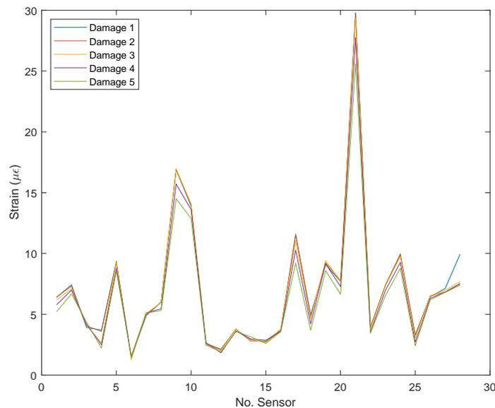
**Figure 9.** Average strain versus sensor number (FBG number) for an excitation frequency of 20 Hz and for the five levels of damage severity.
