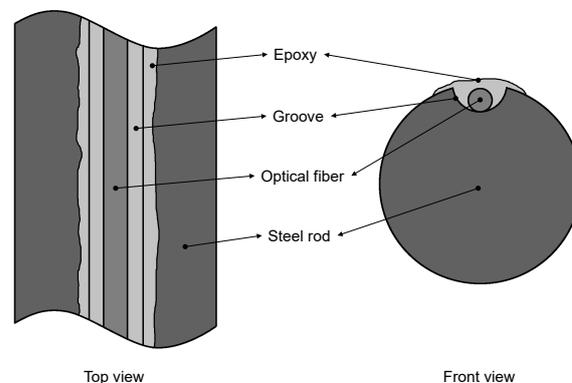
**Figure 3.** Schematic view of reinforcing steel bars instrumented with FBGs.
