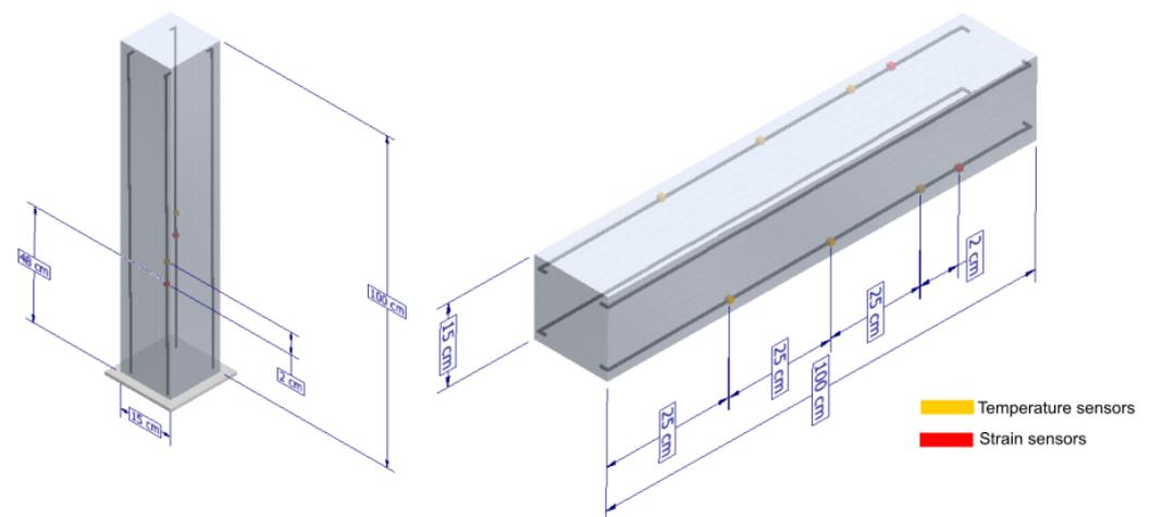
**Figure 4.** Detailed view of sensor location. **Left:** columns. **Right:** beams.
