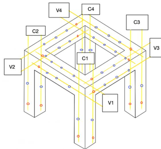
**Figure 2.** Schematic location of fiber optic lines with sensors. Blue dots represent strain sensors and red dots temperature sensors.
