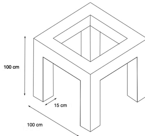
**Figure 1.** General dimensions of the framed structure.
