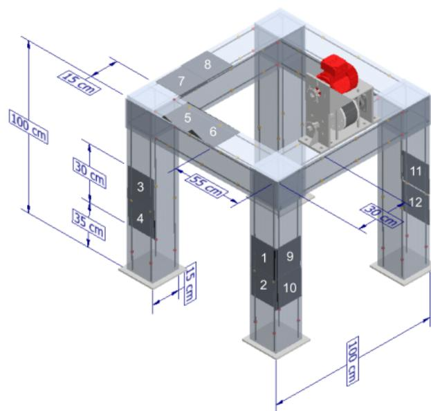
**Figure 6.** Location of artificial positive damages. Yellow dots represent strain sensors and red dots temperature sensors.
