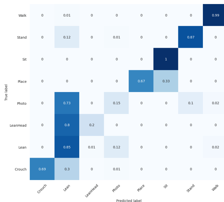
Figure 9. Confusion matrix of the action recognition task on CCTV dataset-split1 performed by the SlowFast network, with darker color indicates higher hit.
