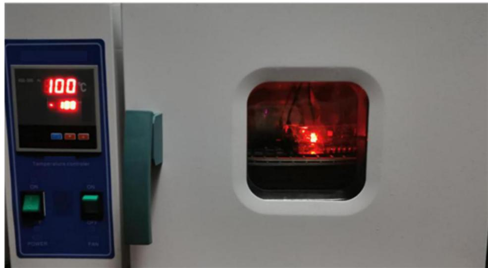
**Figure 4.** Operation state of the high-temperature test chamber.
