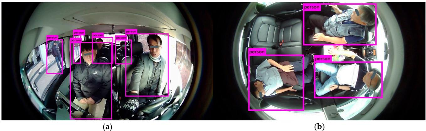
**Figure 13.** A comparison of occupant’s recognition using different positioning of monitoring camera: (a) Occupant’s recognition for FF camera; (b) Occupant’s recognition for RT camera.
