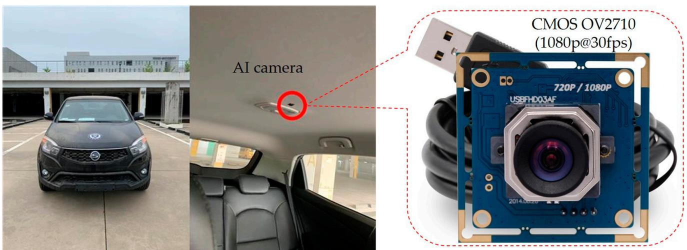
**Figure 4.** A four-seater vehicle is used in the development of DB. The left image depicts the AV used for DB collection, and the AI camera is discerned on the right side of the image.
