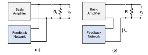
**Figure 6.** Highlighting the physical difference between an output signal from a circuit with a feedback loop and the signal being sensed by the feedback network. (**a**) The output voltage is the same signal that is being sensed by the feedback network, and (**b**) the output voltage is different from the current signal that is being sensed by the feedback network.
