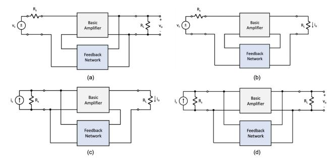
Figure 2. The four noncompliant single-loop feedback topologies incorporated with circuits: (a) voltage-mixing/voltage-sensing, (b) voltage-mixing/current-sensing, (c) current-mixing/current-sensing, and (d) current-mixing/voltage-sensing.
