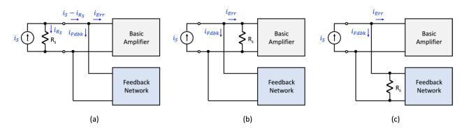
**Figure 5.** Three equivalent current-mixing arrangements; two are compliant with Black's single-loop feedback structure: (**a**) noncompliant, (**b**) compliant option 1, and (**c**) compliant option 2.
