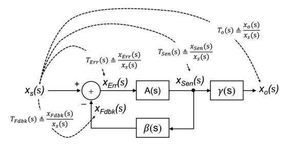
**Figure 8.** Illustrating the intermediate transfer functions associated with a single-loop feedback circuit.
