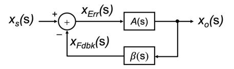
Figure 1. The general form of a negative feedback structure, as first proposed by H. Black.
