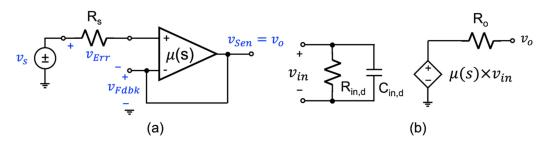
**Figure 9.** Voltage-mixing/voltage-sensing topology: (a) Unity-gain amplifier using an op-amp, and (b) op-amp circuit model with general gain function  $\mu$ (s). The voltage-mixing signal are highlighted in blue.
