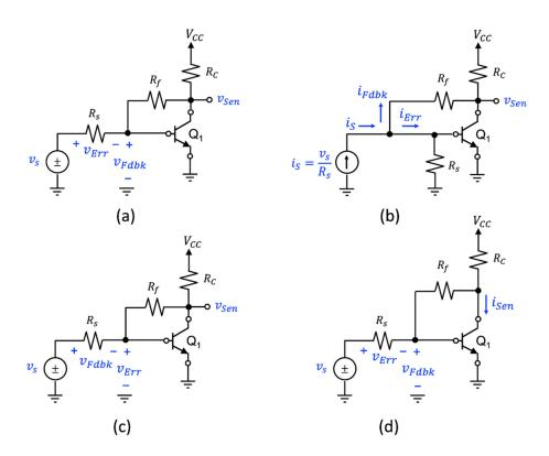
**Figure 14.** Different feedback formulation for a CE BJT amplifier with resistive feedback: (a) voltage-mixing/voltage-sensing compliant arrangement with feedback variable highlighted in blue, (b) through a Norton transformation, the CE amplifier is rearranged into an equivalent current-mixing/voltage-sensing compliant topology, (c) interchanging the feedback and error signal designations, and (d) selecting the sense signal as the collector current rather than the collector voltage.
