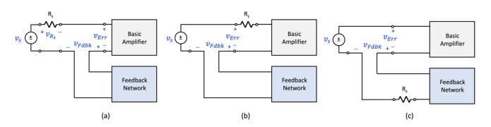
**Figure 4.** Three equivalent voltage-mixing arrangements; two are compliant with Black's single-loop feedback structure: (**a**) noncompliant, (**b**) compliant, and (**c**) compliant.
