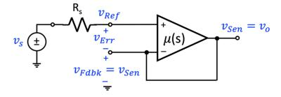
**Figure 11.** A unity-gain amplifier circuit that is to be mapped to the modified single-loop feedback structure of Figure 10. The circuit is the same, but the voltage-mixing variables have been changed.
