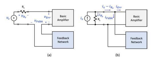
**Figure 3.** Highlighting problem with voltage and current mixing when a source resistance is present. (a) voltage mixing, and (b) current mixing.
