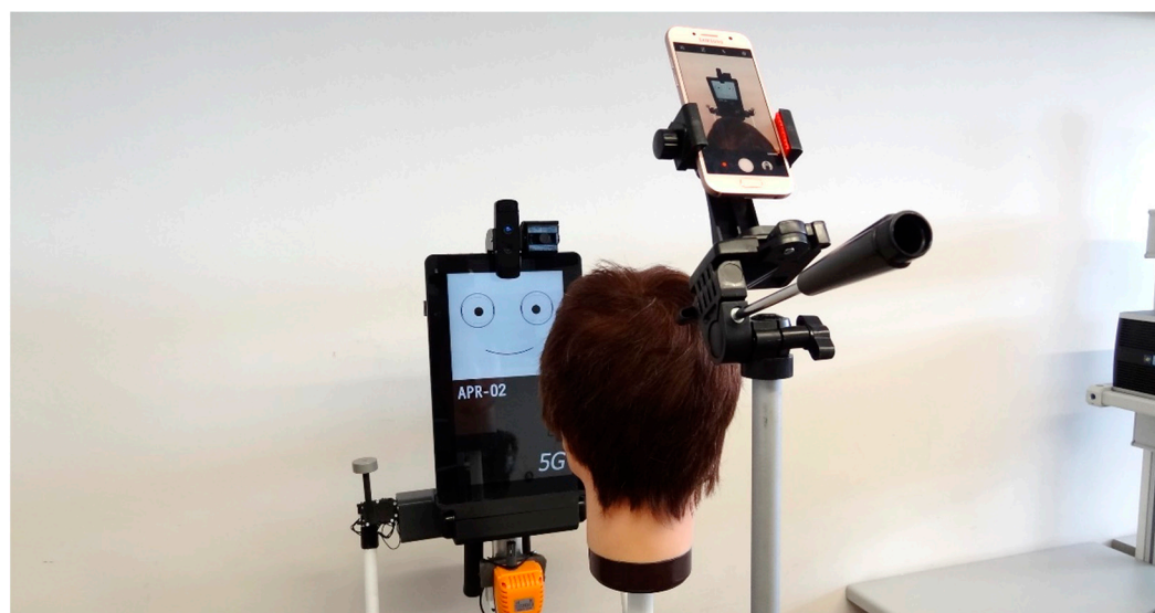
Figure 7. Image of the measurement setup showing the assistance mobile robot, the mannequin head and the camera used to take pictures of the robotic eye-gaze response.
