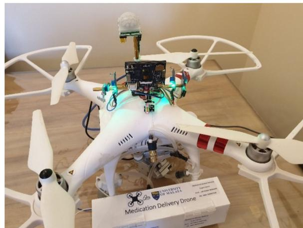
**Figure 1.** Drone with facial recognition and medical delivery box.
