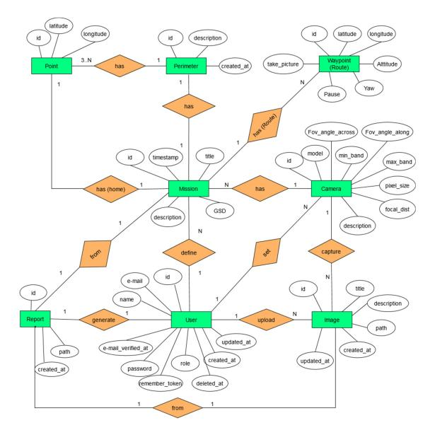
Figure 2. Entity-Relationship diagram of the system database.
