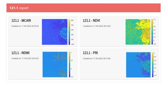
tral image. This visualization is achieved automatically with specific MATLAB functions. Figure 14 shows an example of a visualization of four indexes.
