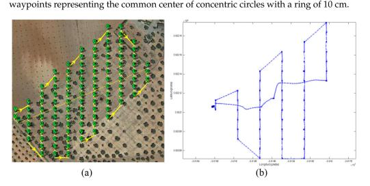
**Figure 16.** (**a**) A mission visualized in Mission-Planner program. (**b**) The actual sub-route recording UAV real GPS waypoints.
