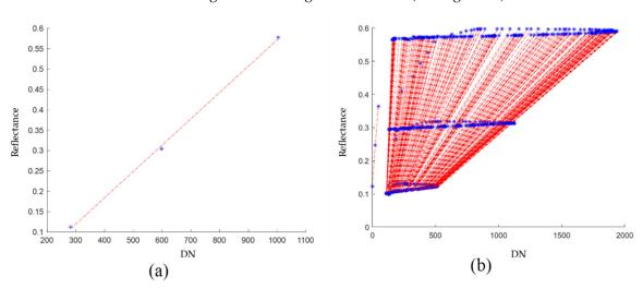
Finally, the parameters of the linear regression that approximates these points for each of the wavelengths in the image are obtained. (See Figure 10).
