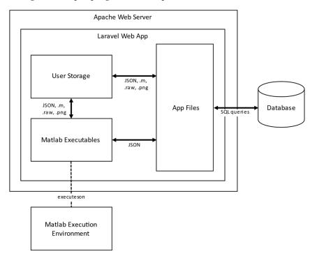
Figure 1. Software architecture and modules organization.
