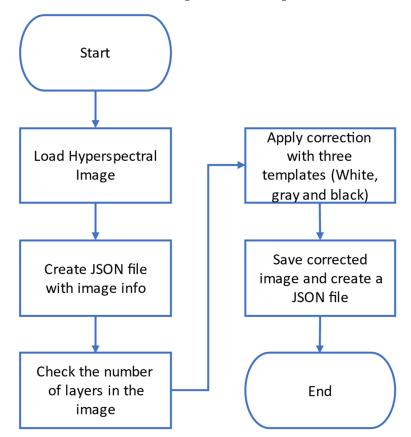
Figure 11. Flowchart followed in MATLAB for multispectral images correction.
