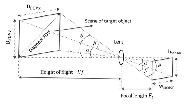
Figure 5. Field of view and camera parameterization.
