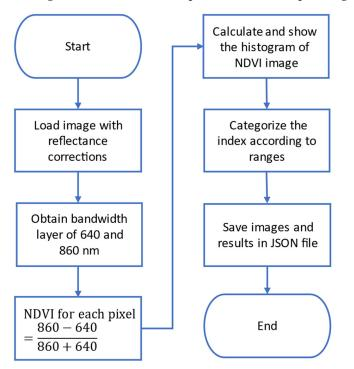
Figure 12. Flowchart of the main steps in the NDVI index processing.
