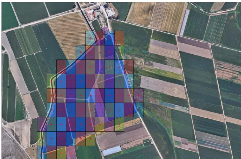
**Figure 6.** Waypoints obtained from a tessellation process without overlap between tiles. Route starts from the bottom to the top and from the left to the right.
