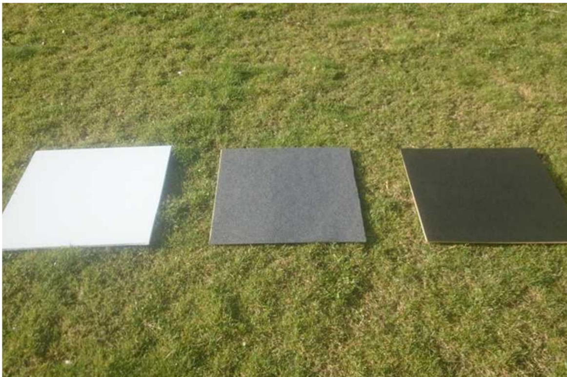
**Figure 9.** Templates for reflectance calibration, (Image from MosaicMill).
