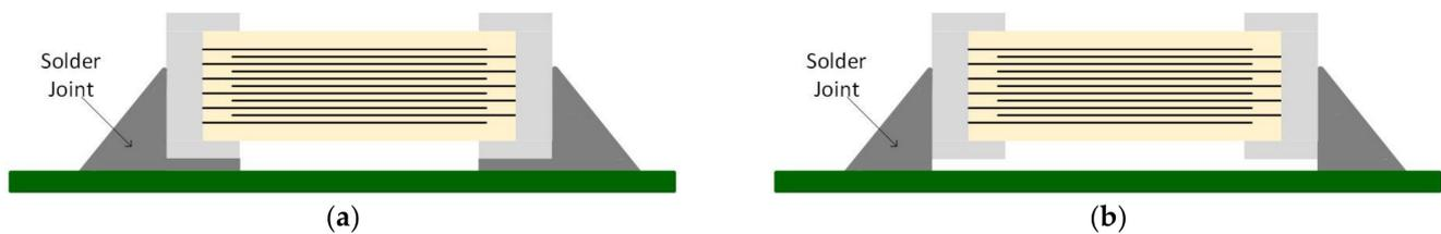
**Figure 13.** MLCC soldering (a) Classical soldering; (b) Proposed soldering.
