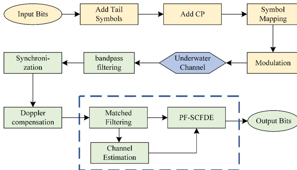
Figure 1. Block diagram of the CPM with the PF-SCFDE UWA communication system.
