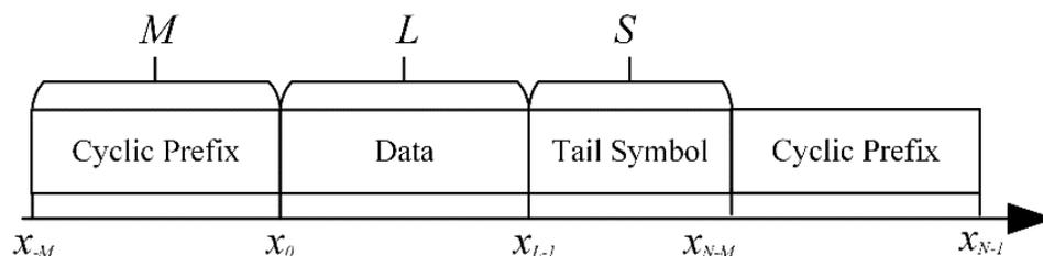
Figure 2. Complete frame structure.
