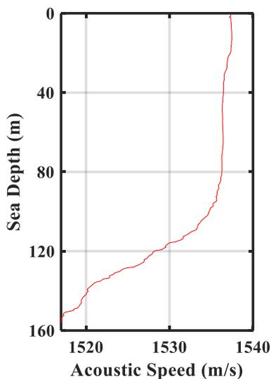
Figure 10. Measured sound velocity.
