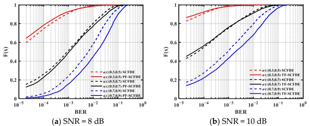
Figure 5. BER cumulative distribution function for GMSK.
