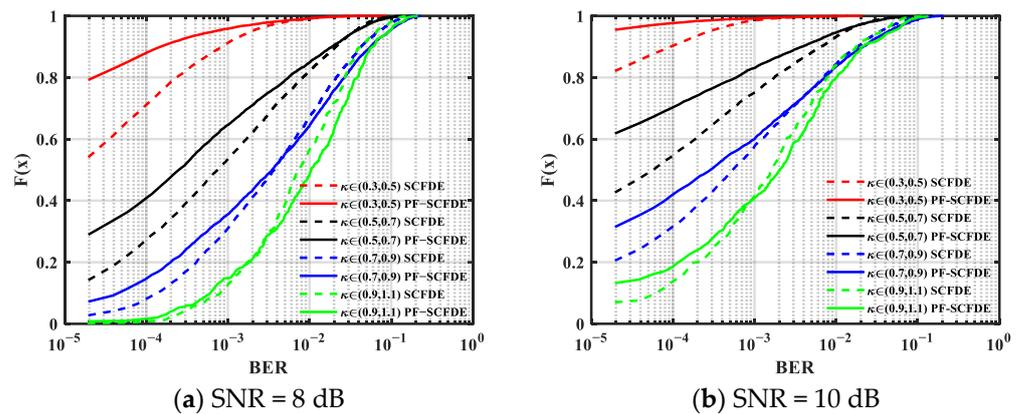
Figure 4. BER cumulative distribution function for MSK.
