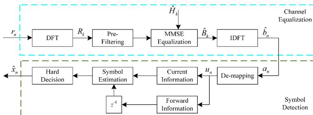
Figure 3. CPM receiver with PF-SCFDE.
