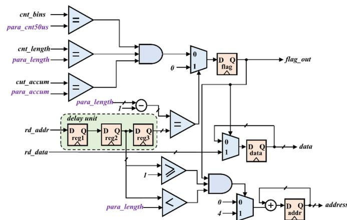
Figure 7. The logic structure diagram of the output module.
