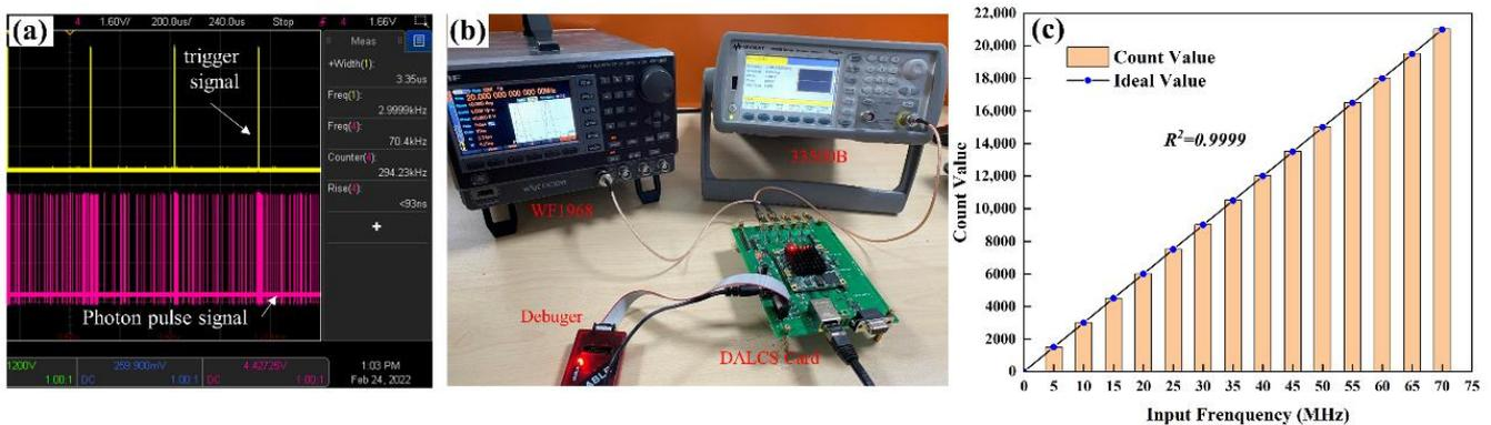
**Figure 10.** Signal test: (a) Laser and PMT module output signal; (b) Test environment; (c) Count linearity.
