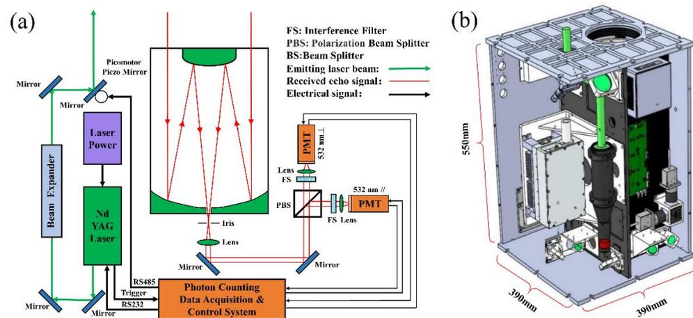
**Figure 1.** Lidar sensor system: (a) schematic diagram and (b) internal structure diagram.
