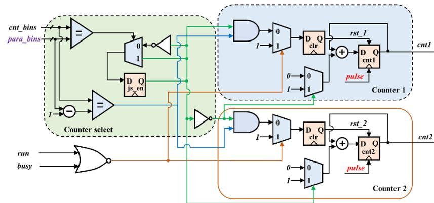
Figure 6. The logic structure diagram of the counting module.
