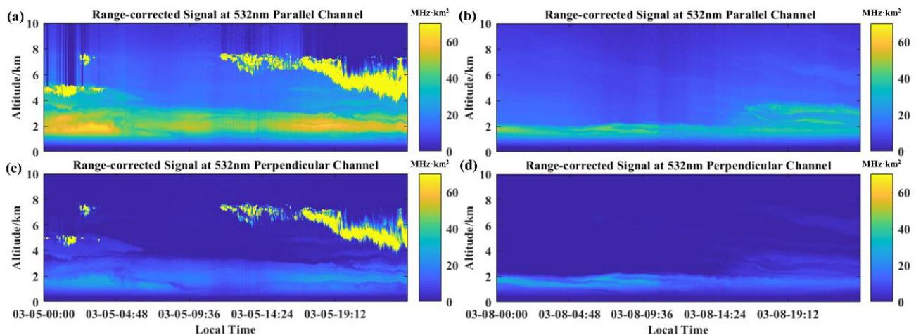
**Figure 13.** Range-corrected signal profiles in different weather: (a) 532 nm parallel Polarization channel on 5 March 2022; (b) 532 nm vertical Polarization channel on 5 March 2022; (c) 532 nm parallel Polarization channel on 8 March 2022; (d) 532 nm vertical Polarization channel on 8 March 2022.
