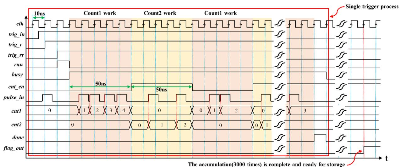
**Figure 8.** Main logic signal diagram of the acquisition system.
