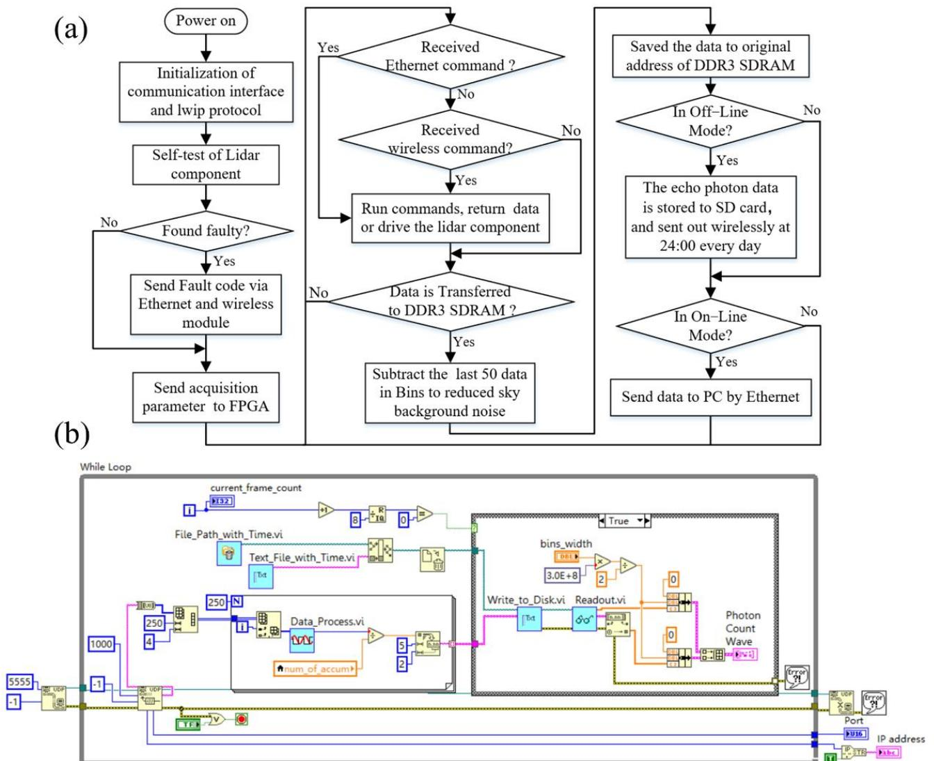
**Figure 9.** Software design: (a) embedded program flow chart; (b) the main program of the upper computer.
