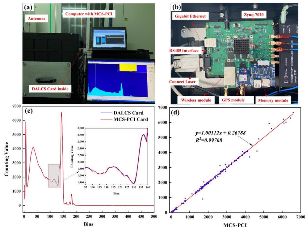
Figure 12. Actual test: (a) Lidar test platform; (b) DALCS Card; (c) comparison of DALCS and MCS-PCI; (d) linear fitting of DALCS and MCS-PCI.
