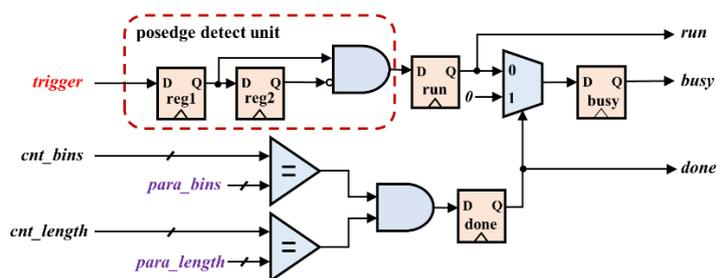
Figure 5. The control module logic structure diagram.
