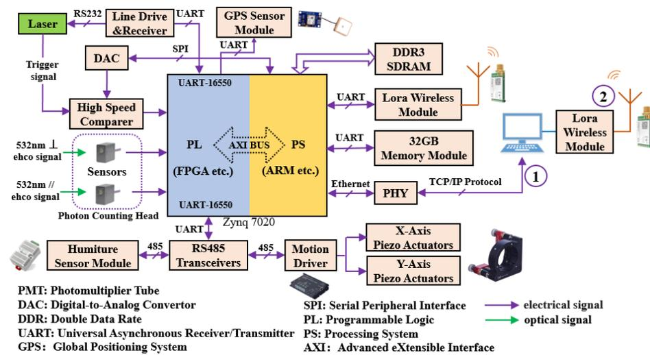
Figure 2. Block diagram of DALCS hardware structure.
